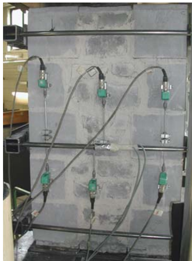
Fig. 6 Wall repaired with steel rods
